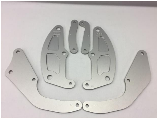
BAR Engineplates set for 85cc Junior Speedway bikes Made to fit Suzuki, Honda and TM engines.
