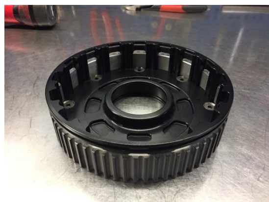
BAR Beltdrive project BAR Basket fitted with GG beltdrive Steel sprocket
